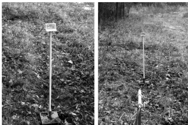
Figure 2. Measuring position: a) HE charge on a stand; b) pressure sensor on a stand.
