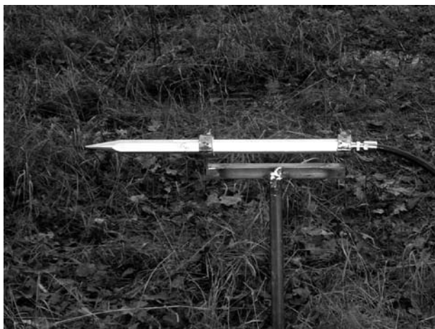
Figure 1. PCB 137A23 sensor installed in the measuring position.
