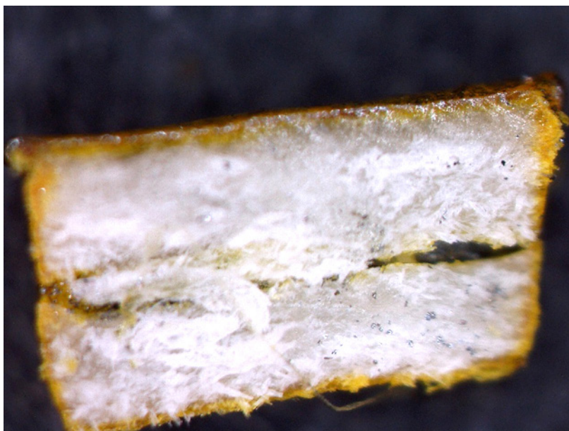
Figure 1. Image of M1 propellant grain fracture; orange layer corresponds to the thickness of the modified layer
