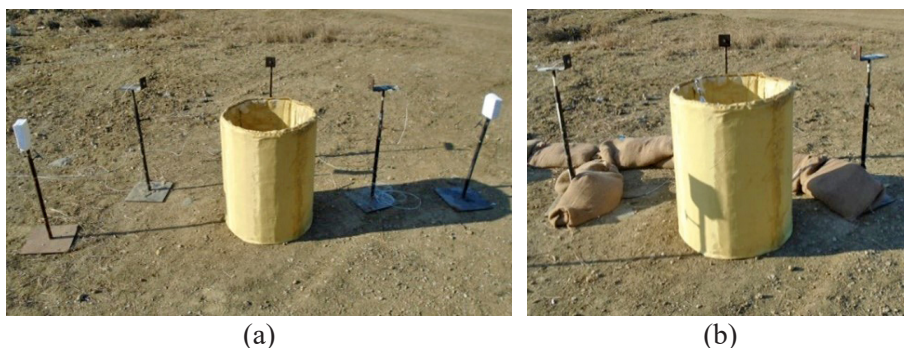
Figure 6. Experimental setup for 800 g C4 detonation inside container
