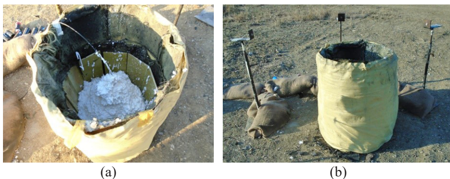
Figure 14. Shaving foam filled around steel cased charge (a) and experimental setup (b)
