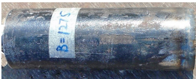
Figure 7. Steel cased charge (pipe-bomb)
