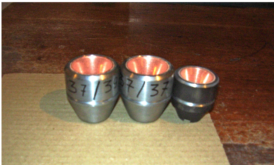
Figure 3. Experimental samples of the tested conical SCs
