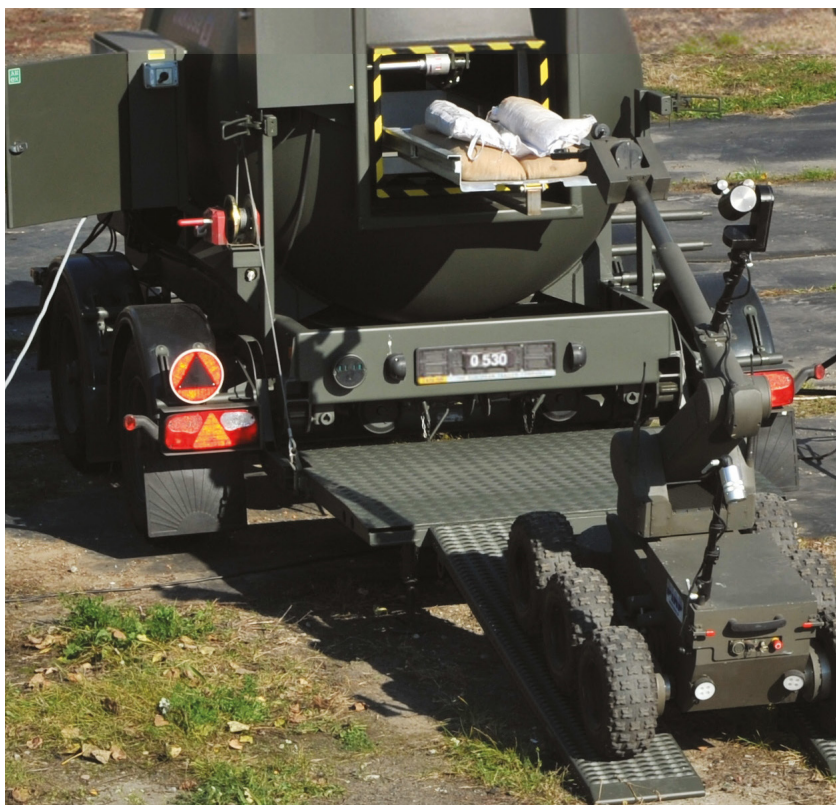
Figure 7. The Wiktoria ventilated container for transporting explosives [11]
