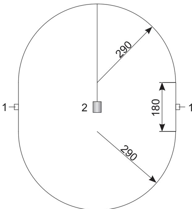
**Figure 1.** Diagram of the explosion chamber with installed pressure sensors and attached explosive charge:
