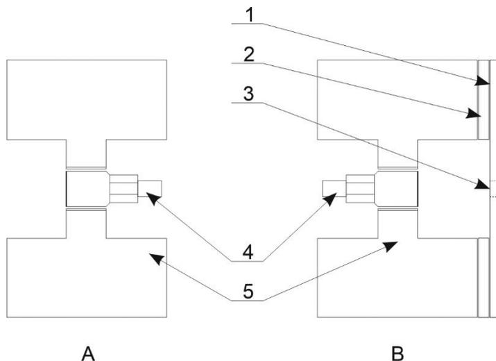
**Figure 2.** Diagram of two socket types prepared for fitting pressure sensors: 1 – membrane, 2 – teflon spacer, 3 – passage duct, 4 – pressure sensors, 5 – steel pressure sensor fitting sockets
