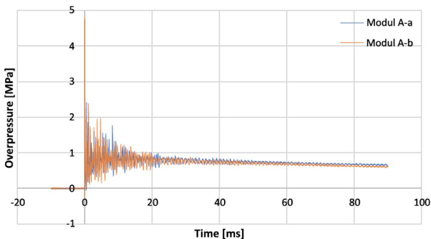
**Figure 3.** Recording overpressure changes in the chamber with the sensors fitted using module A
