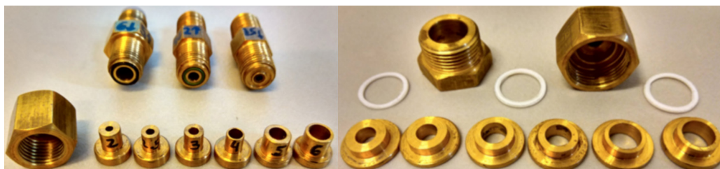
Figure 3. Set of test membrane mounting components for testing diameter series: 2, 2.5, 3, 4, 5, 6, 8, 10 and 12 mm
