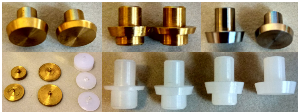
Figure 2. Nozzle closure concepts tested using adhesive bonding
