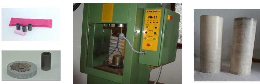
Figure 10. Station for pressing pyrotechnic products and product examples
