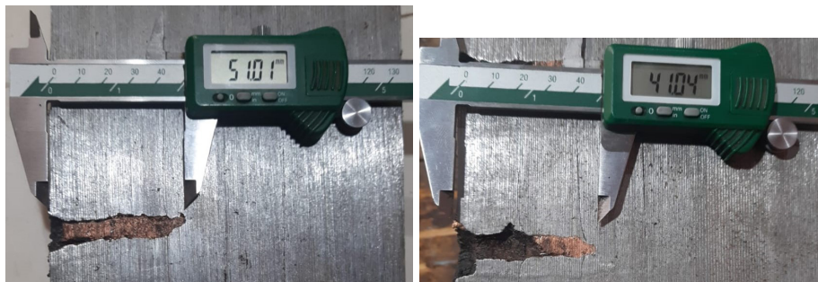
Figure 14. The experimental penetration for both the jet (left) and the EFP (right)
