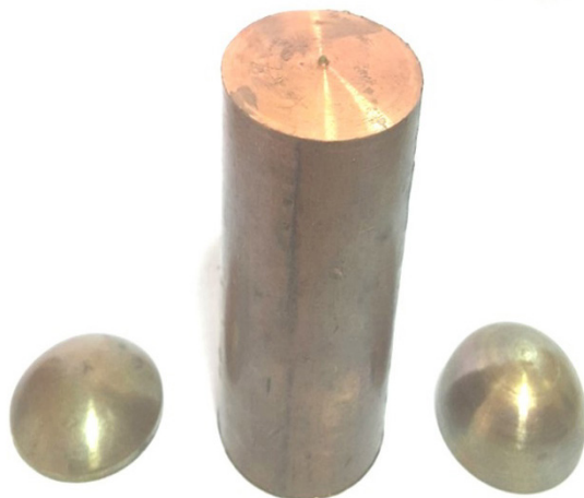
Figure 2. Dimensions and geometry of hemispherical (a), dish-shaped liner (b), manufactured hemispherical and dish-shaped liners (c)
