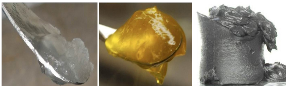
Figure 1. Enhanced viscosity, and stability of metalized gel propellant [16, 17]
