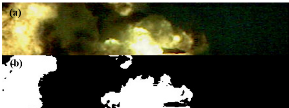
Figure 11. Process of high-speed photographic image: (a) original image and (b) binarized image
