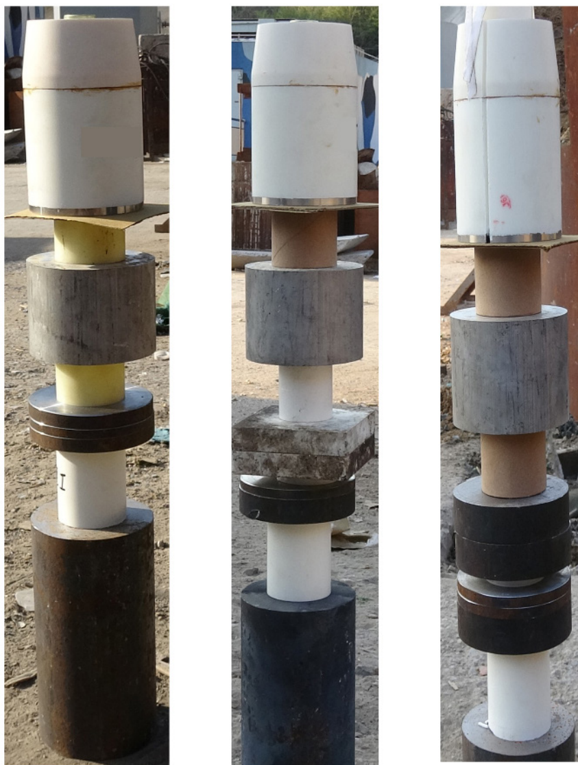
Figure 3. Images of: – Configuration 1, with only 10 mm outer steel container wall (a), – Configuration 3, which utilizes 40 mm ceramic add-on protection (b), and Configuration 4, which employs 40 mm steel protection at 10 mm gap from container 10 mm container wall (c)
