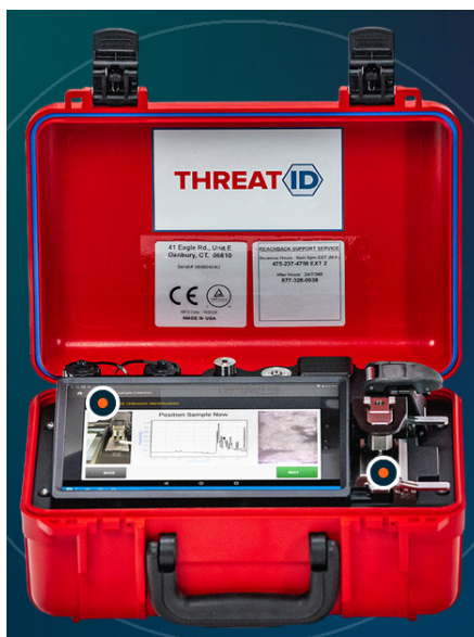
Figure 10. ThreatID FTIR spectrometer by 908 Devices [75]
