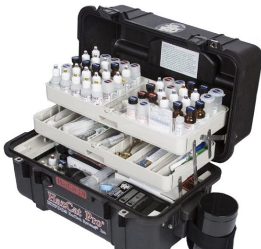
Figure 17. HazCat 2.0 colour test kit for hazardous material identification
