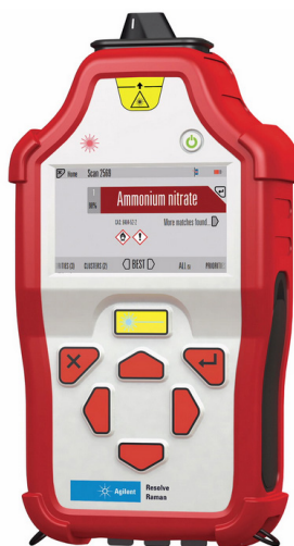
Figure 2. Resolve Handheld SORS by Agilent Technologies [40]
