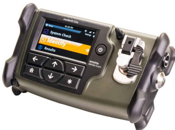
Figure 8. HazMatID Elite FTIR spectrometer by Smith's Detection [69]
