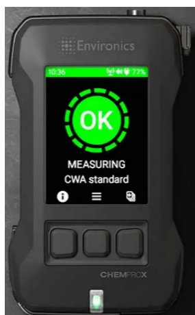
Figure 20. ChemProX detector by Bertin Environics [98]
