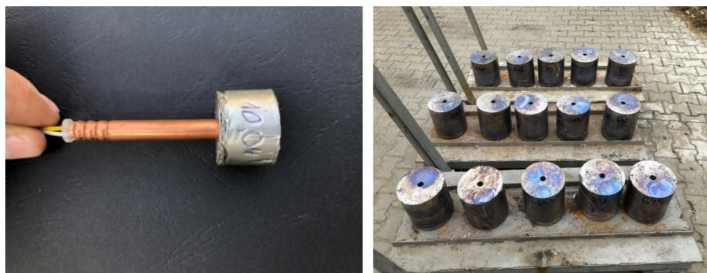
Figure 2. Foil-wrapped explosive sample with detonator (left) and blocks before the test (right)
