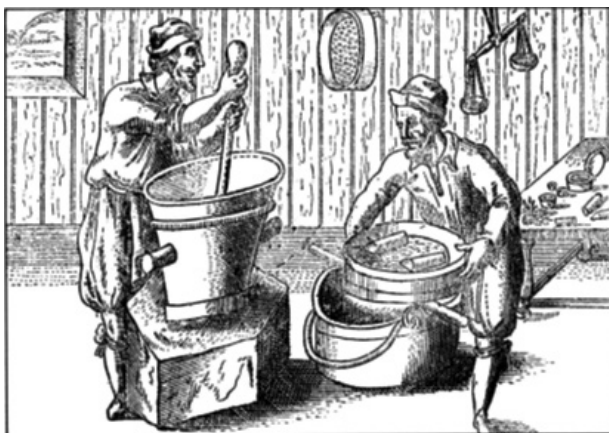
Figure 2. The process of grinding the black powder components in a mortar (on the left) and mashing the paste through a sieve (on the right) [16, 17]
