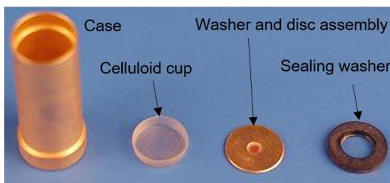
**Figure 1.** Engineering sketch **Figure 2.** Cartridge components
