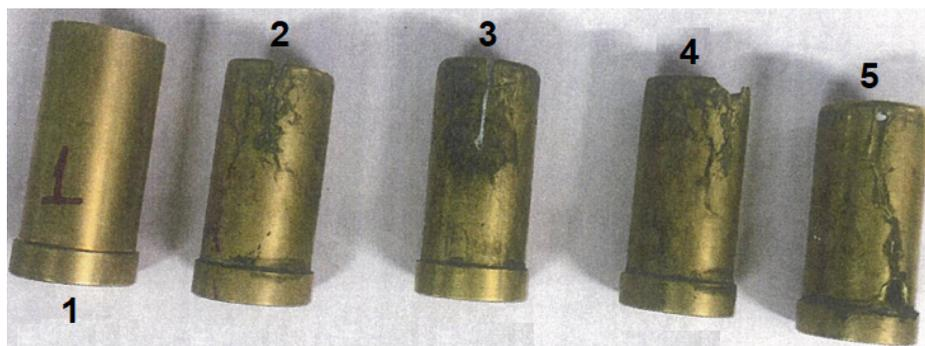
**Figure 4.** Visual examination of brass cartridge cases after firing
