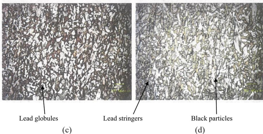
**Figure 6.** Micro-structure of an unfired brass cartridge case indicating two-phase structure ( $\alpha$  and  $\beta$  phases) and black particles and stringers of lead at 200X
