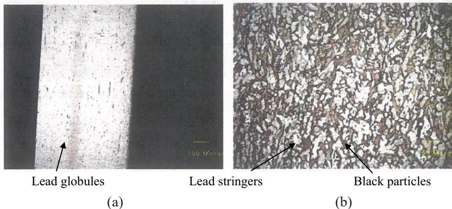
**Figure 6.** Micro-structure of an unfired brass cartridge case indicating two-phase structure ( $\alpha$  and  $\beta$  phases) and black particles and stringers of lead at 100 X
