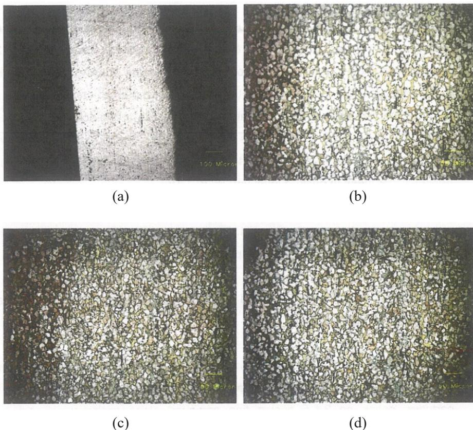
**Figure 8.** Burst brass cartridge case (crack and holes at mouth and base), at 200X, two-phase structure  $\alpha$  and  $\beta$ , equiaxed  $\alpha$  grains and black lead particles (in longitudinal section): unetched (a), and etched: – base (b), – middle (c) and – mouth (d)
