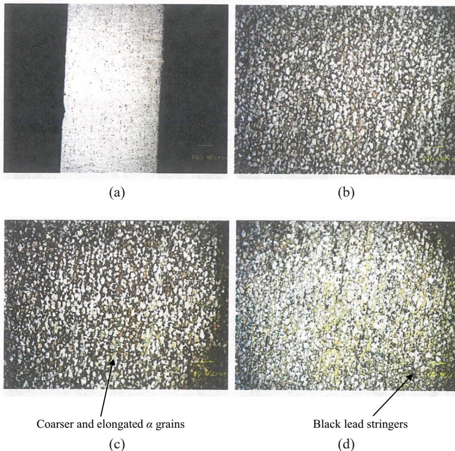
**Figure 7.** Micro-structure, at 200X, of a fired brass cartridge case indicating two-phase structure, slightly coarser and elongated  $\alpha$  grains in the matrix of  $\beta$  and black lead stringers in longitudinal section: – unetched (a), and etched: – base (b), – middle (c) and – mouth (d)
