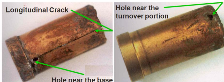
**Figure 5.** Enlarged view of cartridge case indicating a longitudinal crack and a burst
