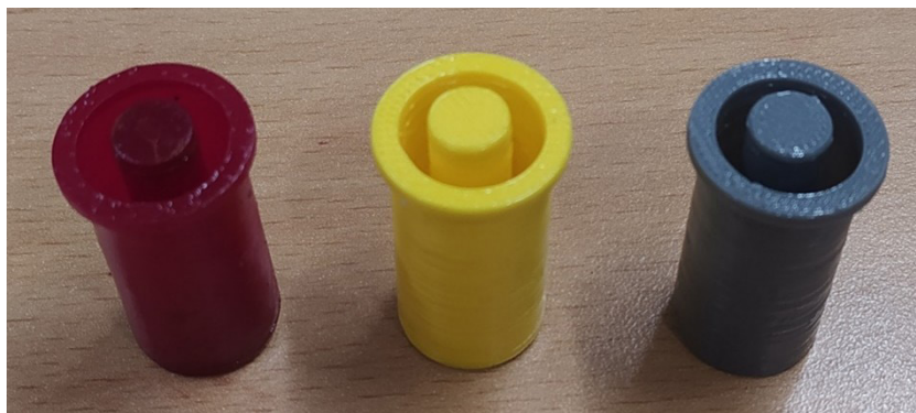
Figure 1. Individual moulds were made from three different materials: a water-soluble resin, ABS, and HIPS
