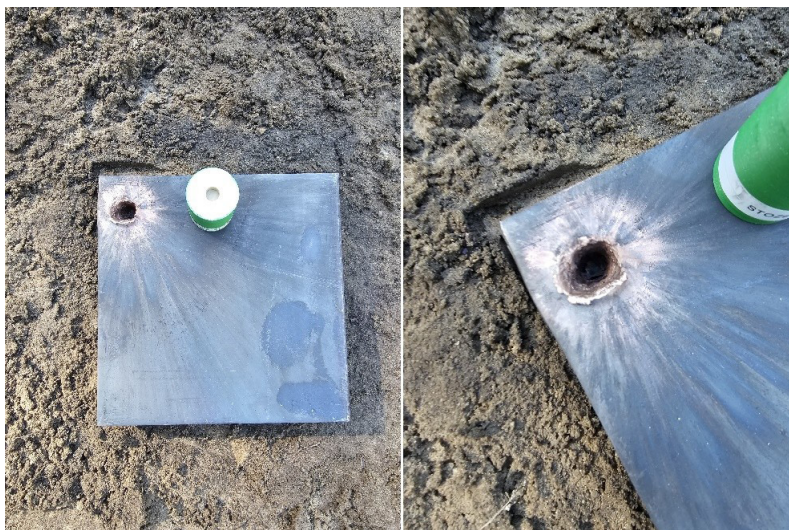
Figure 7. Examples of results of the entry openings after a shot with a shaped charge during steel plate penetration tests
