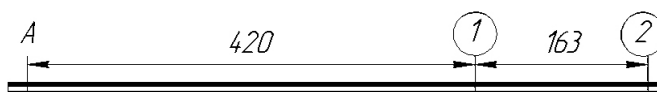
Figure 1. Scheme of experiments with a detonating shock tube: A – point of application of the initiating electric explosion, 1 and 2 – piezoelectric sensors
