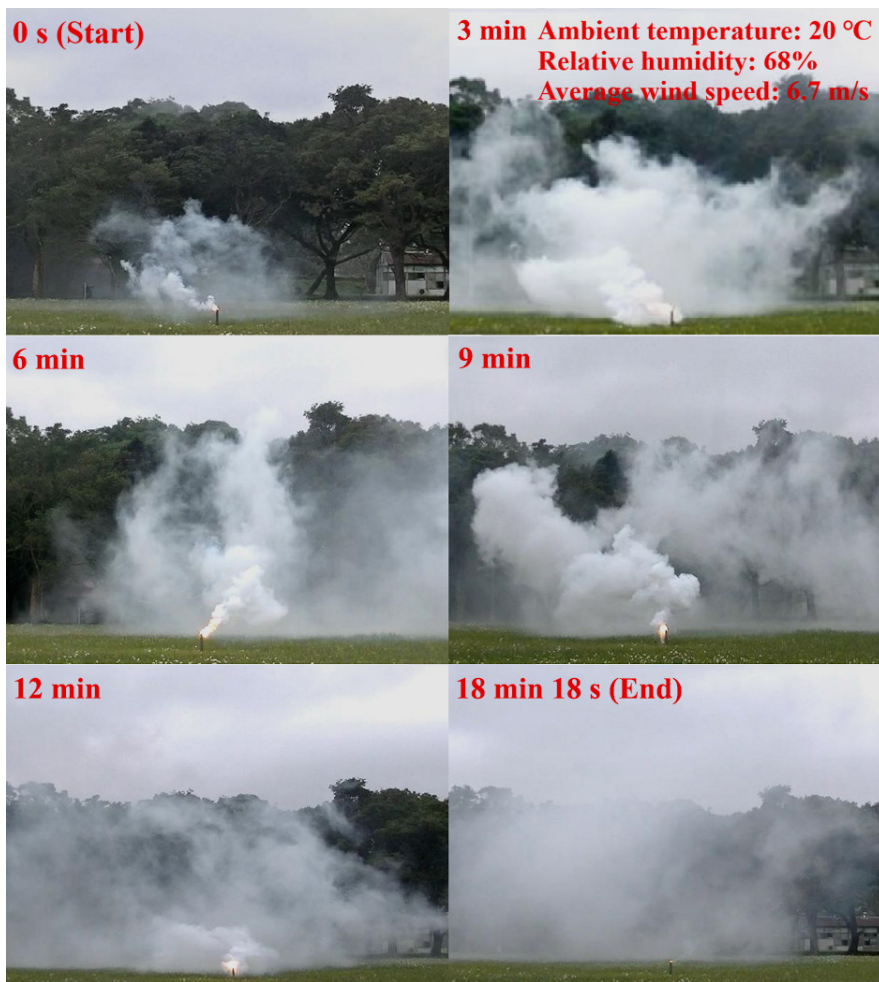
Figure 13. A series of consecutive images of combustion phenomenon taken by digital video camera for full-size RP smoke candle with \text{KNO}_3 as oxidizer
