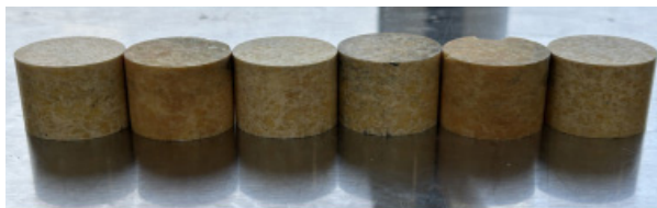
Figure 6. Photograph of TNT charges
