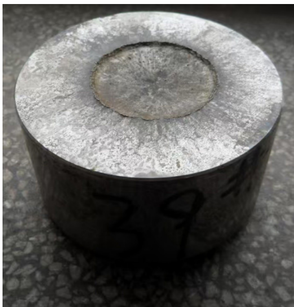
Figure 11. Schematic of the blast velocity test setup: pre-test photograph of a columnar sample (a) and the scheme of the detonation velocity test (b)
