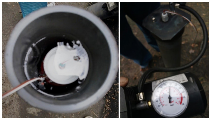
Figure 3. Explosive charge in a water-filled pipe and application of pressure using compressor
