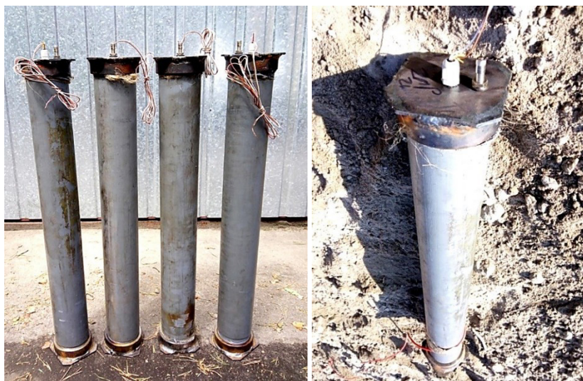
Figure 4. View of the charged and pressurized explosive samples
